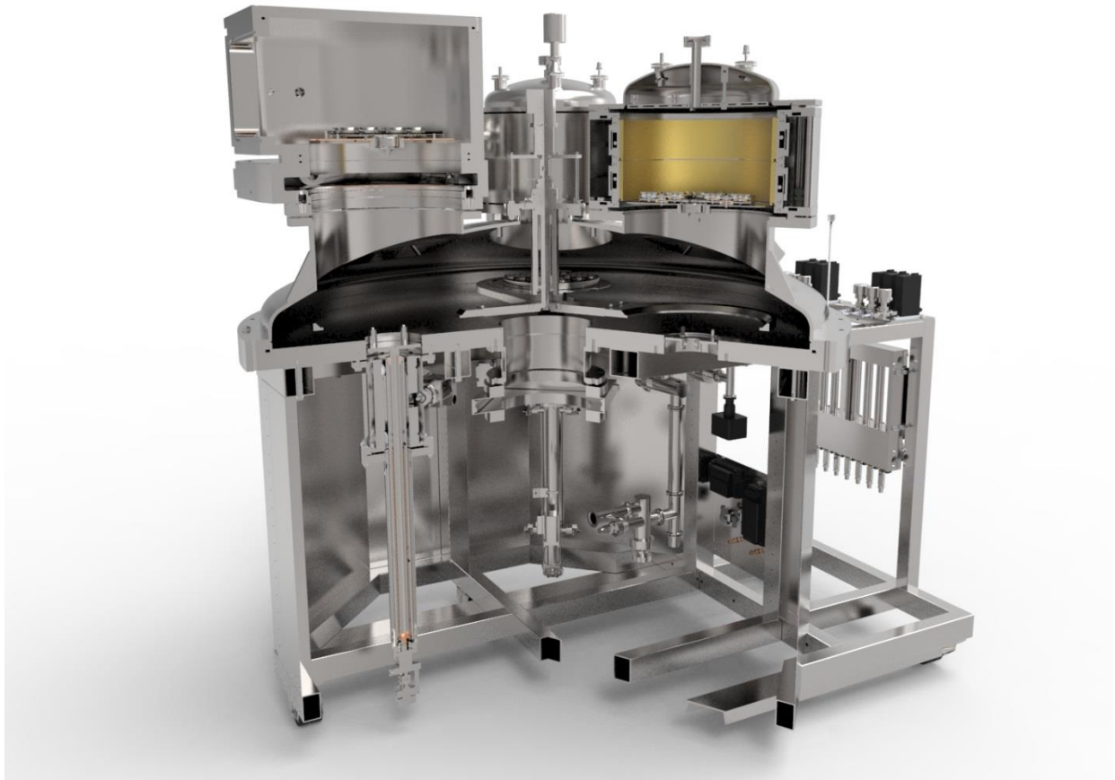
Figure 2. Cutaway view of the system layout showing the load lock on the left and sputtering cathode on the right.
